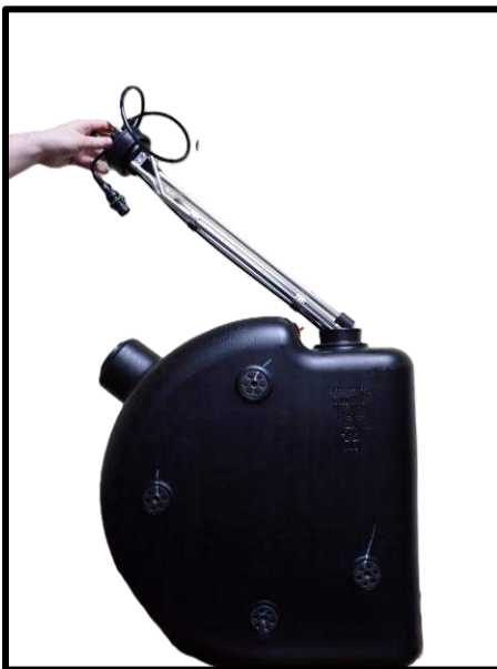
Figure 2.3 Installation of MFHU into DEF tank
