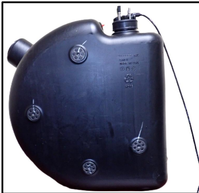
Figure 2.4 Installation of MFHU into DEF tank
