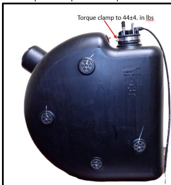
Figure 2.5 Installation of Hose Clamp
