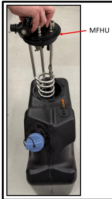
Figure 2.4- Multifunction Head Unit Installation
